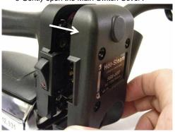
7- Remove 2 wires screws.
