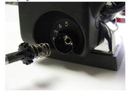
4-Remove the Temperature Dial Housing.
