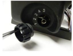
5-Remove Main Switch Cover screws (3)
