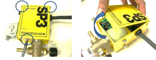
2- Remove the nut with a wrench and remove the Solenoid Valve from the box.
