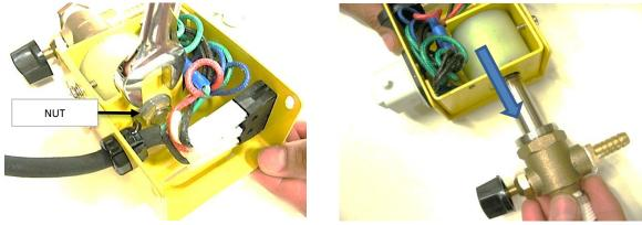
3- Hold the Body (use a vise to hold the body if necessary) and remove the Steam Pipe with a wrench. Remove and replace the Plunger&Spring Set and the Gasket from the Steam Pipe.
