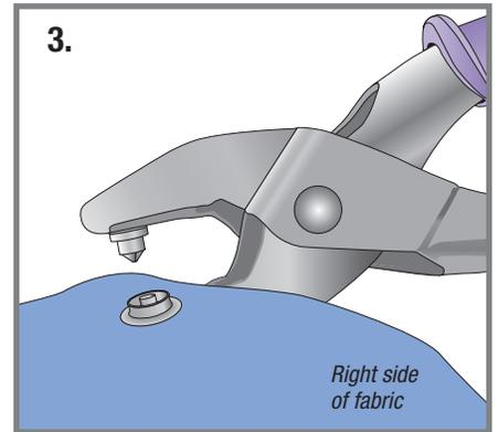
4. Squeeze pliers firmly to apply stud and post. Check for tightness; squeeze again, if necessary.
