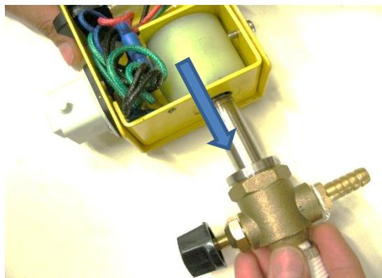
3- Hold the Body (use a vise to hold the body if necessary) and remove the Steam Pipe with a wrench. Remove and replace the Plunger&Spring Set and the Gasket from the Steam Pipe.
