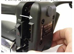
7-Remove Thermal Fuse screws (2) and replace Thermal Fuse
