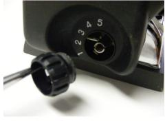
5-Remove Main Switch Cover screws (3)
